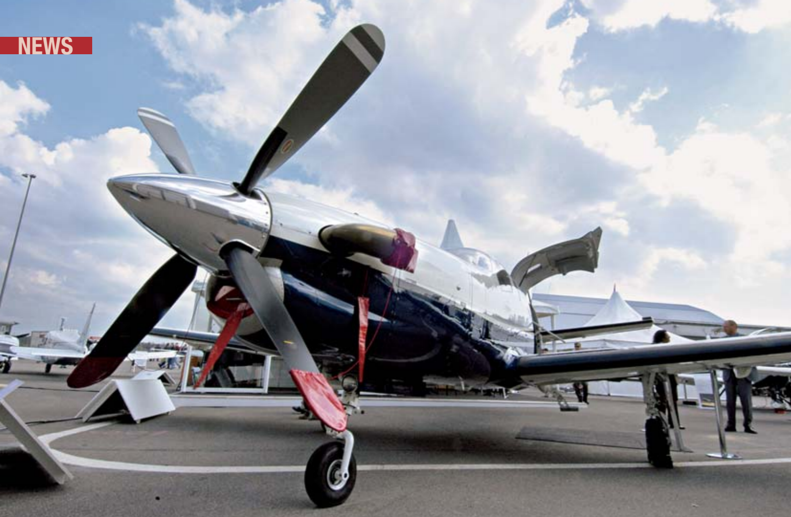
At a cruising speed of 300 knots, the Socata TBM 700 is the world's fastest single-engine turboprop
