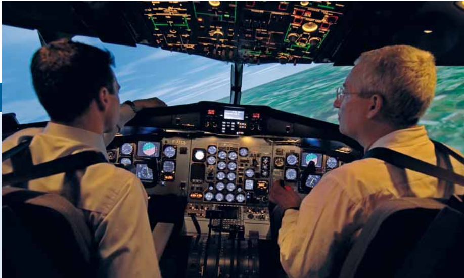
ATR's new full flight trainer (FFT) creates an almost perfect illusion of flight at a significantly lower cost than a full flight simulator (FFS)
