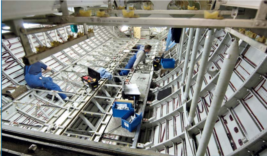
Vertical struts are installed to reinforce the upper deck
