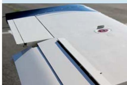
Spoilers on the top of the wing assist the short ailerons
