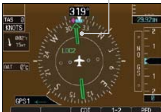
Figure 2-34 Auto-Slewing HSI with Localizer Backcourse Loaded and Shown with the Corresponding Approach Plate
