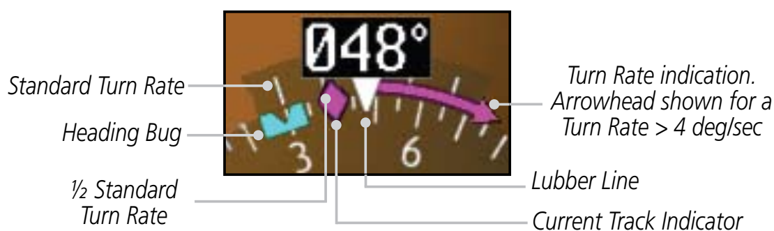
Figure 2-27 Turn Rate Indicator and Trend Vector
