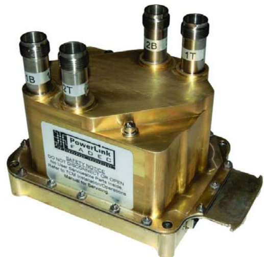
PowerLink FADEC IOF-240-B installed in certified Liberty XL2 Aircraft
