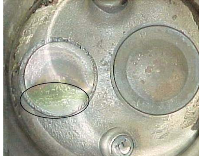
Burned Exhaust Valve
