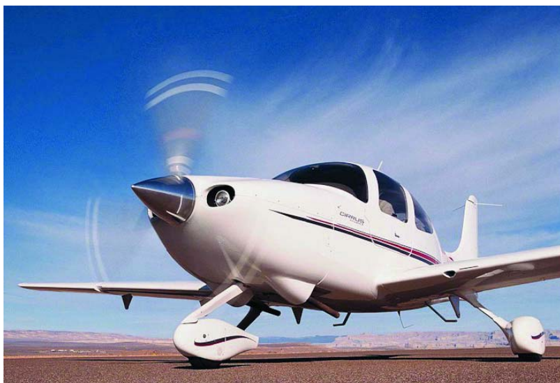
Figure 6. Cooling Air Openings in a Typical Well Designed Installation.
