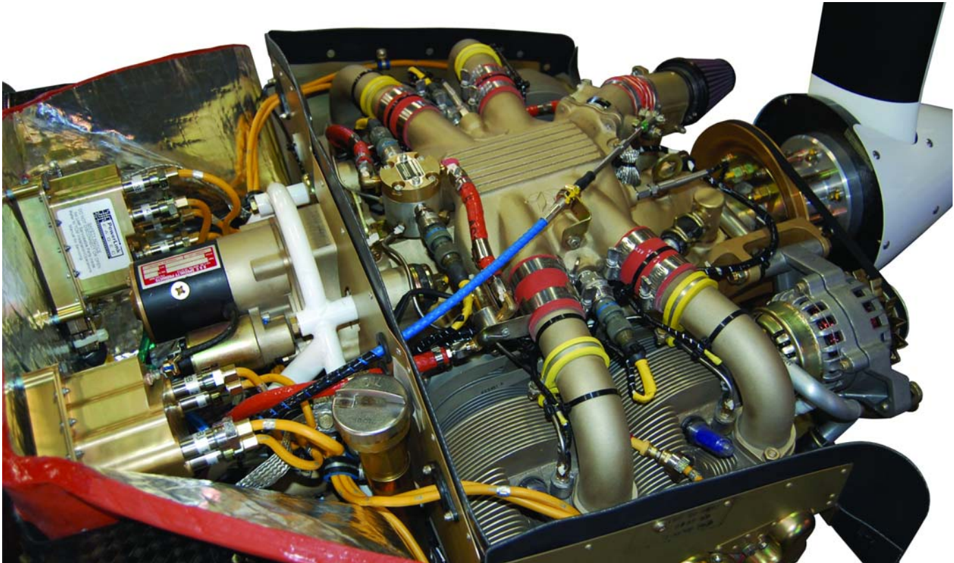
PowerLink FADEC IOF-240-B installed in certified Liberty XL2 Aircraft
