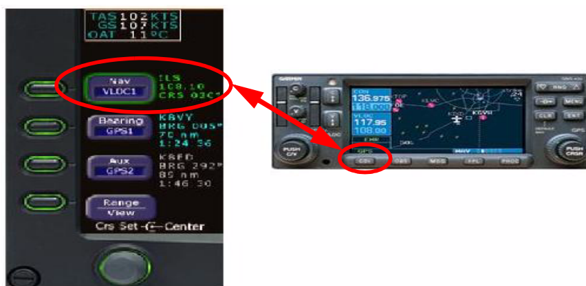
Figure 9. Setting CDI Scale on EXP5000's HSI
