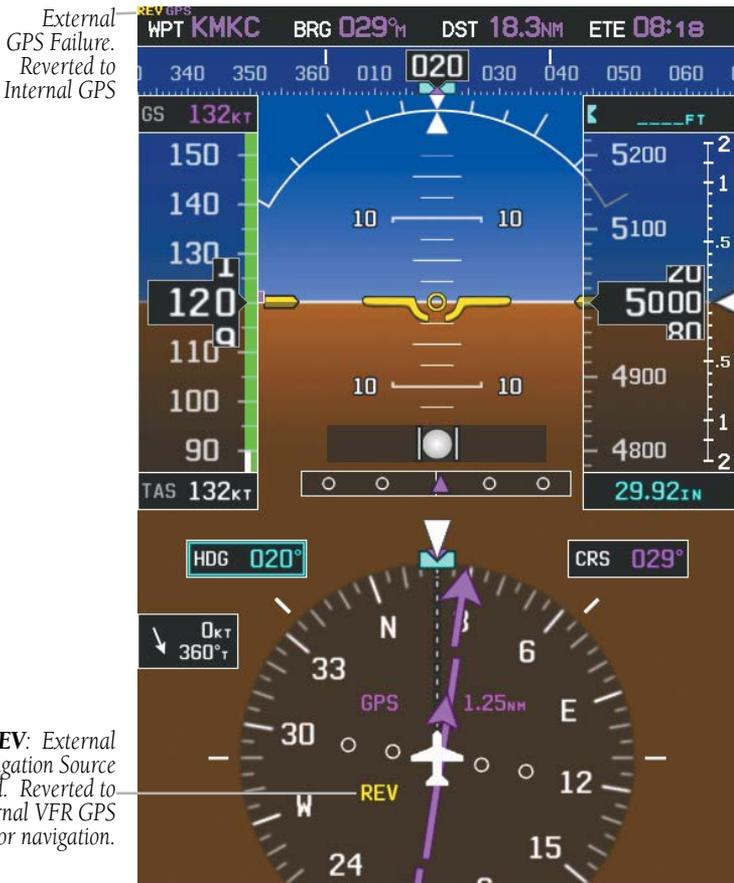
**External GPS Navigation Failure**
