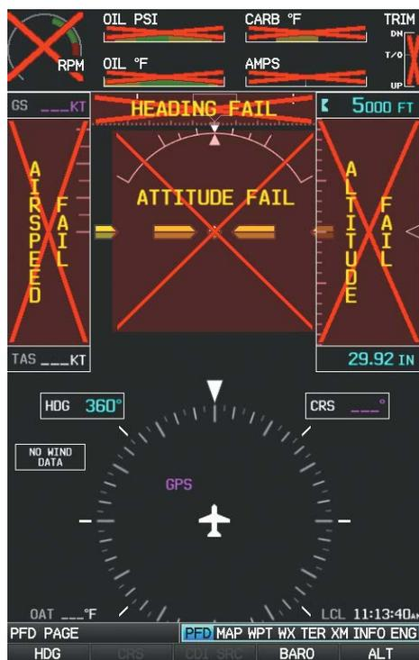
G3X System Failure Annunciations
