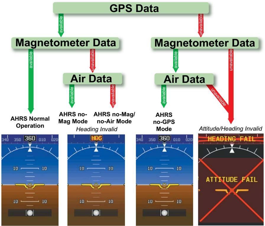
Loss of GPS, magnetometer, or air data inputs is communicated to the pilot by message advisory alerts. Any failure of the internal AHRS inertial sensors results in loss of attitude and heading information (indicated by red 'X' flags over the corresponding flight instruments). If the G3X senses that the magnetic heading measurement is valid, but possibly outside of the internal accuracy limits, the numeric heading value on the PFD is displayed in yellow.
