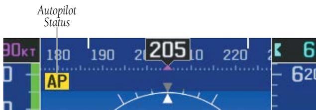
Autopilot Manually Disengaged
