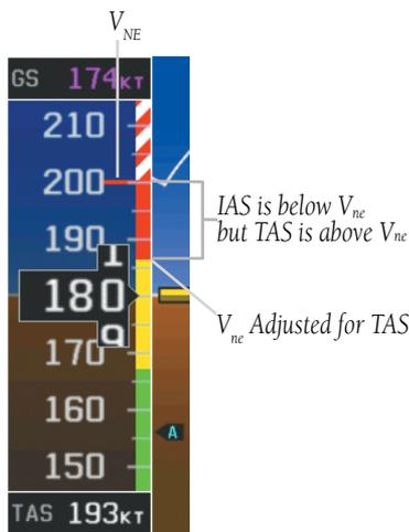
V<sub>ne</sub> Adjusted for True Airspeed
