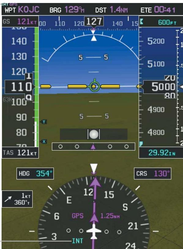
**INT:** The pilot has elected to use the internal GPS navigation source instead of the external GPS navigation source.
