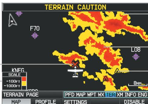
Yellow Terrain is Between the User-defined Caution Elevation and 100 ft Below the Aircraft
