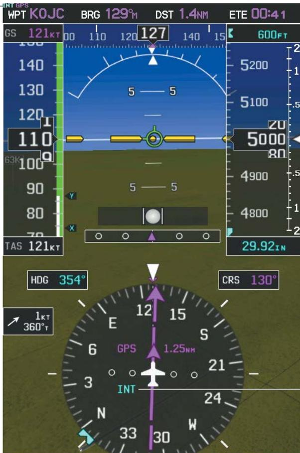
*INT: The pilot has elected to use the internal GPS navigation source instead of the external GPS navigation source.*
