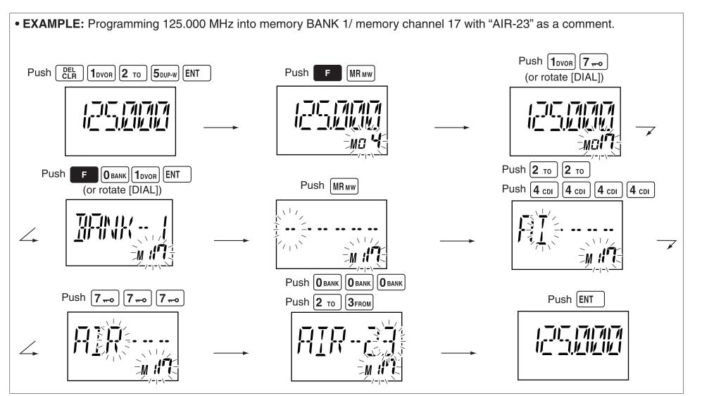
**NOTE:** Push **F**, then push [0•BANK], and then rotate [DIAL] to select the BANK number, if desired. Push [CLR•DEL] to exit the BANK selection mode.
