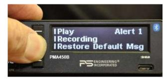
Hold the center button to record a new message using the pilot's microphone Pressing the bottom button will replace the user-stored message with the factory message. In the case of Alert 1, it is a simple chime sound.
