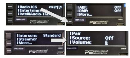
**NOTE**: During the time that the Streamer module is in the pairing process, BT1 is disabled, so music and telephone will not be available. When paired, a Bluetooth "OUT" symbol (a small flag in the symbol) will appear in the
