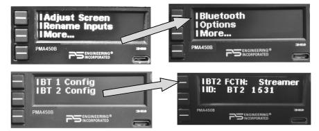
To pair the PMA450B PS Streamer with a compatible device, access the streamer menu from Radio-ICS  $\rightarrow$  More  $\rightarrow$  Streamer  $\rightarrow$  Config  $\rightarrow$  Pair. Now, turn on the desired device and initiate the pairing on the device as well.
