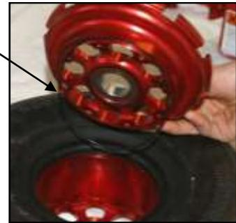
**6** Remove the tyre from the 2 other parts of the wheel, as detailed below.
