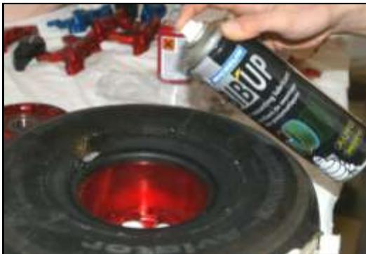
Spray tyre mounting lubricant between the tyre and the wheel.
