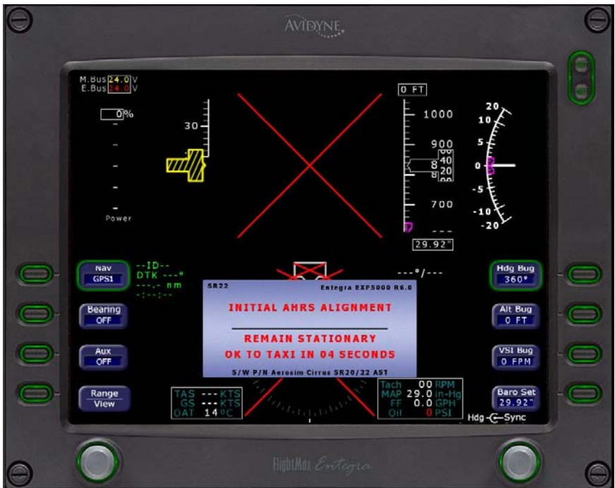
Fig. 2-3. PFD Display, INITIAL AHRS ALIGNMENT Message
