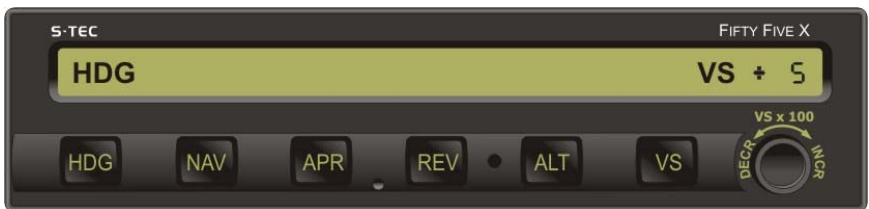
Fig. 3-18. AP Display, HDG and VS Modes Engaged, PFD Failure
