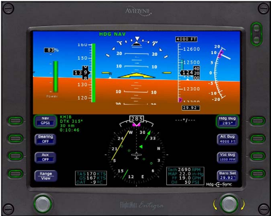
Fig. 3-9. PFD Display, HDG Mode Engaged, NAV Mode Armed
