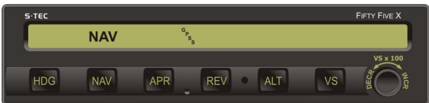
Fig. 3-10. AP Display, GPSS Mode Engaged
