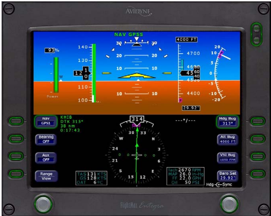
Fig. 3-11. PFD Display, GPSS Mode Engaged
