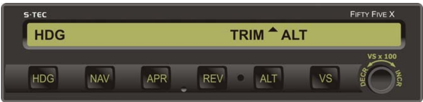
Fig. 3-22. AP Display, HDG and ALT HOLD Modes Engaged, Autotrim in Progress
