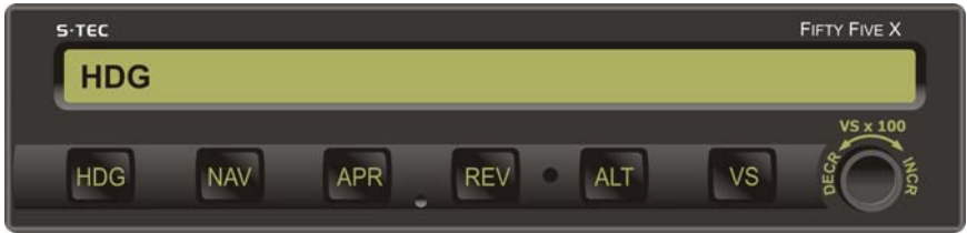
Fig. 2-8. AP Display, HDG Mode Engaged (Pre-Flight)
