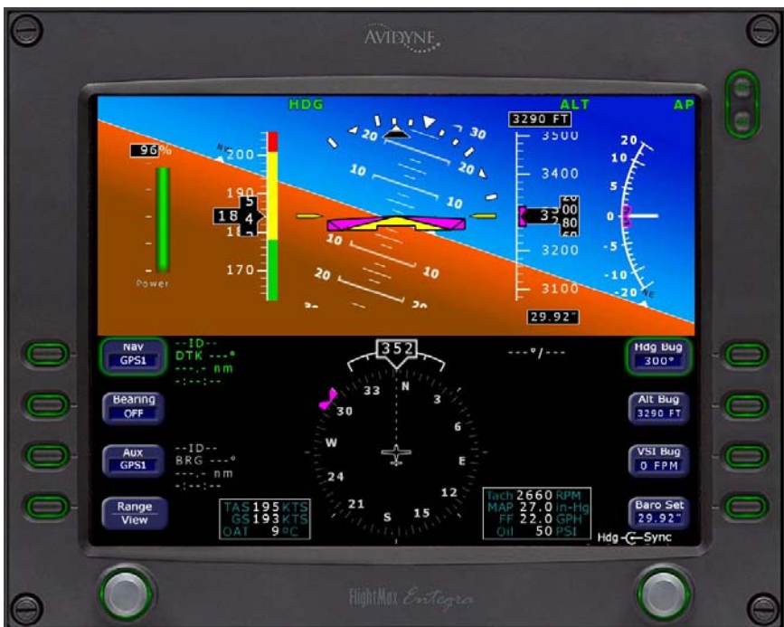
Fig. 3-46. PFD Display, HDG and ALT HOLD AP Modes Engaged
