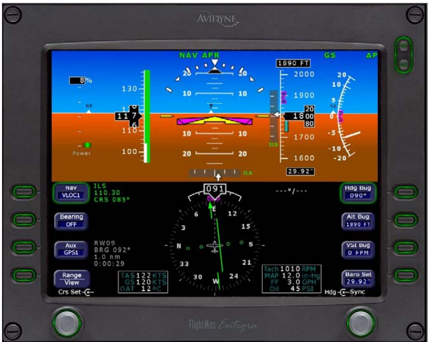
Fig. 3-28. PFD Display, NAV, APR, and GS Modes Engaged
