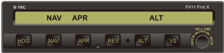
Fig. 3-23. AP Display, NAV, APR, and ALT HOLD Modes Engaged
