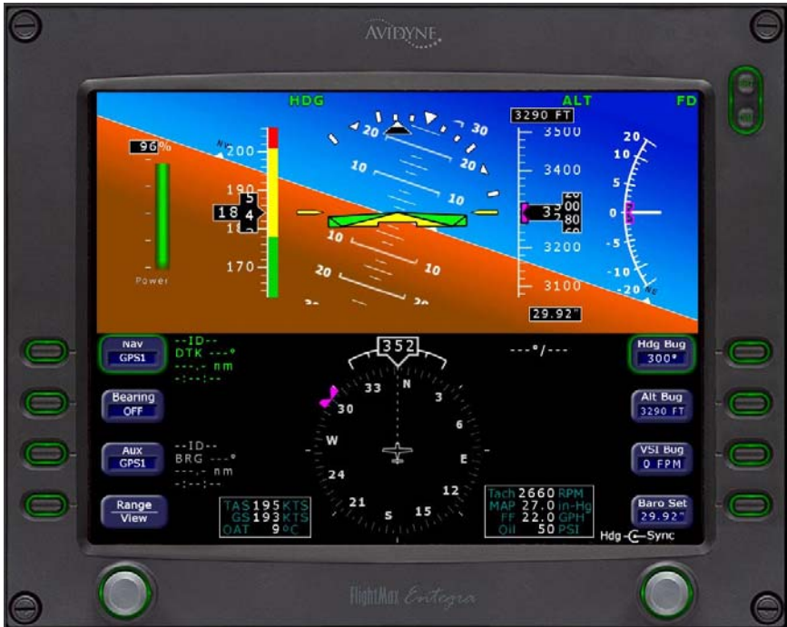
Fig. 3-47. PFD Display, FD Only Mode Engaged
