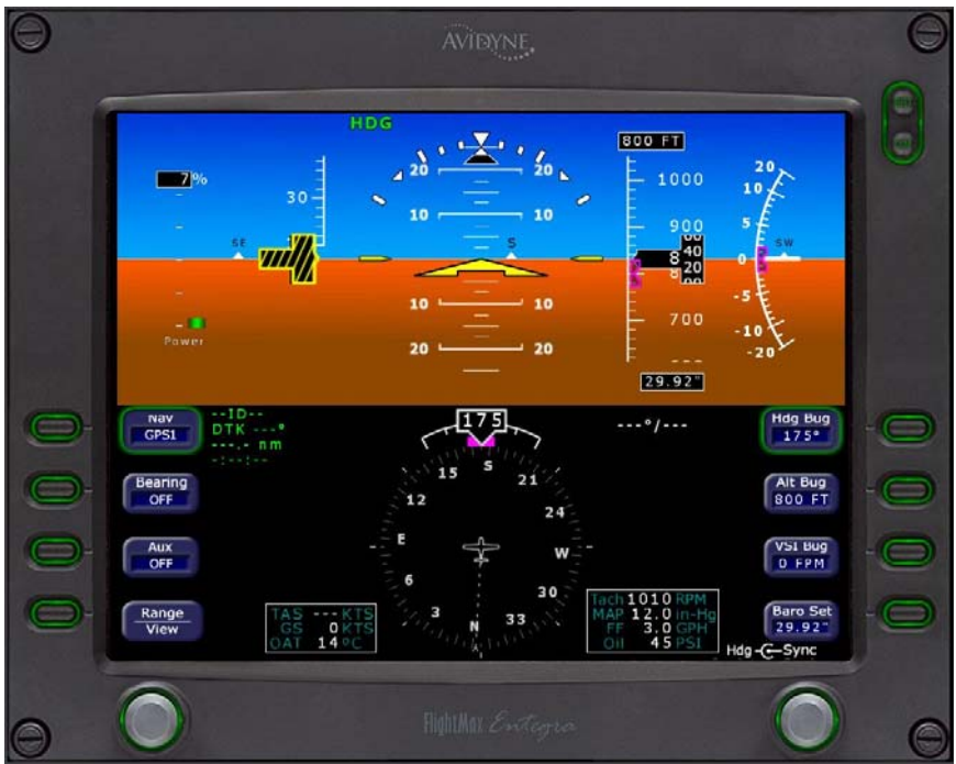
Fig. 2-9. PFD Display, HDG Mode Engaged (Pre-Flight)
