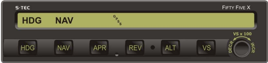
Fig. 3-12. AP Display, HDG Mode Engaged, GPSS Mode Armed
