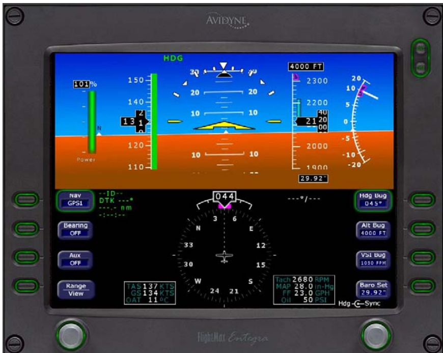
Fig. 3-2. PFD Display, HDG Mode Engaged
