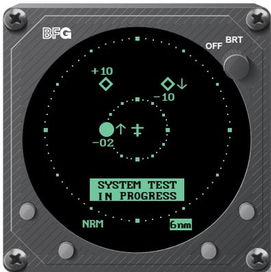
Figure 2-6. Operator-Initiated Test Screen
