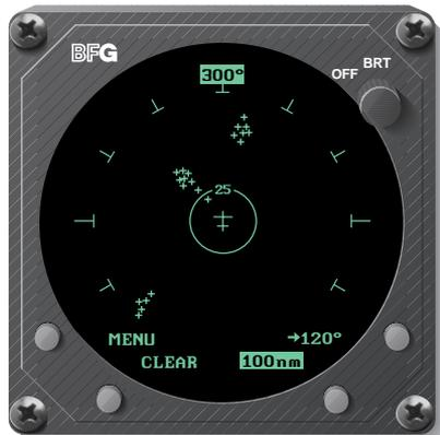
Figure 1-3. Display with Typical STORMSCOPE Screen (Optional)
