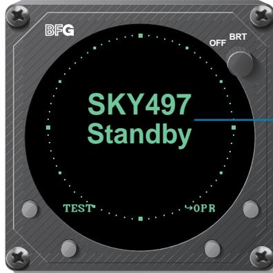
When in standby, the SKY497 does not transmit interrogations or track intruder aircraft. Press the button labeled →OPR to begin tracking intruder aircraft.
