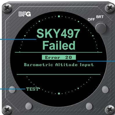
Error 20 indicates that the barometric input is missing or invalid. Once valid barometric input returns, this screen goes away and normal operation resumes. All other errors are unrecoverable, in which case you can switch into optional STORMSCOPE mode, or turn off the SKY497.
